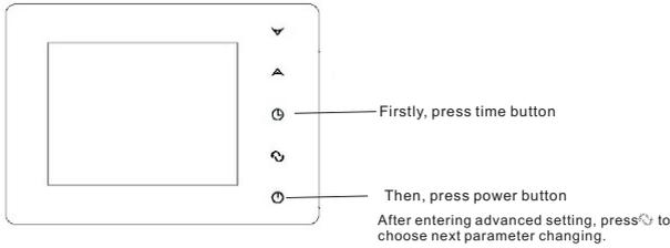
In the state of power-off, long press and hold then press into advanced setting mode. Then press to set relative item.
