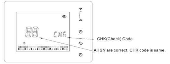
The fourth step, after SN is finished setting, if CHK Code is the same with bar code, it is correct. If not consistent, it is not correct. Please input again.
