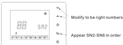
The third step, every time pressing once , it will appear SN2, SN3, SN4, SN5 and SN6 in order. Refer to second step, press or to modify.
