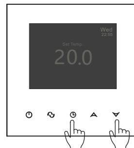
When turning on or off, press the time button and down button simultaneously to enter the green light energy-saving mode. The thermostat is working normally, but there will be a faint display.
