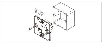
4) Re-mount the front cover via snap-fit connection.
